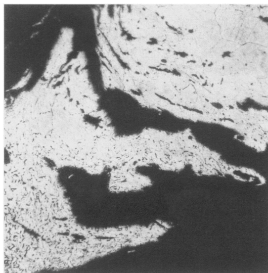
Figure 53. Sample from burgonet in Figure 52 ( \times 95 ). Ferrite, slag inclusions, and a little, partly spheroidized pearlite
