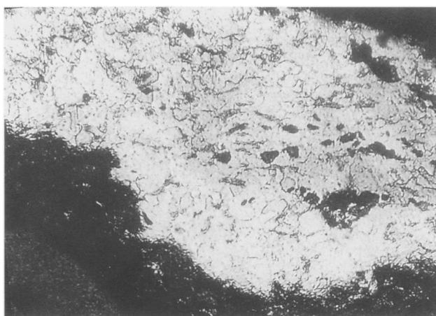
Figure 15. Sample from pauldron in Figure 14 ( \times 200 ). Ferrite and slag inclusions
