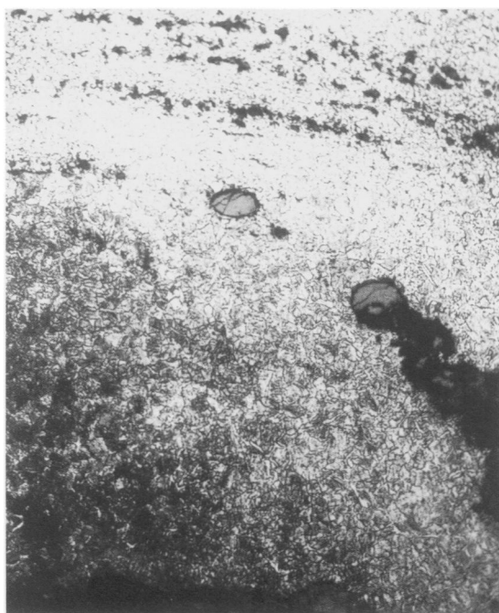
Figure 25. Sample from lower plate of left cheekpiece of burgonet in Figure 24 ( \times 115 ). Pearlite and ferrite with some large iron oxide inclusions
