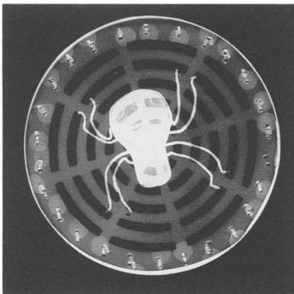
Figure 13. Radiograph of silver-and-gold earflare frontal in Figure 12 (photo: author)
