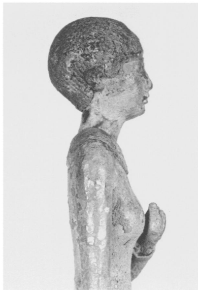
Figure 14. Detail of "carved" corrosion on the statuette
