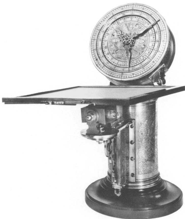
5. Hodometer signed by Christoph Trechsler the Elder and dated 1584, German (Dresden). Gilded brass, H. 16½ in. (42 cm.). Dresden, Mathematisch-Physikalischer Salon (photo: Mathematisch-Physikalischer Salon)
