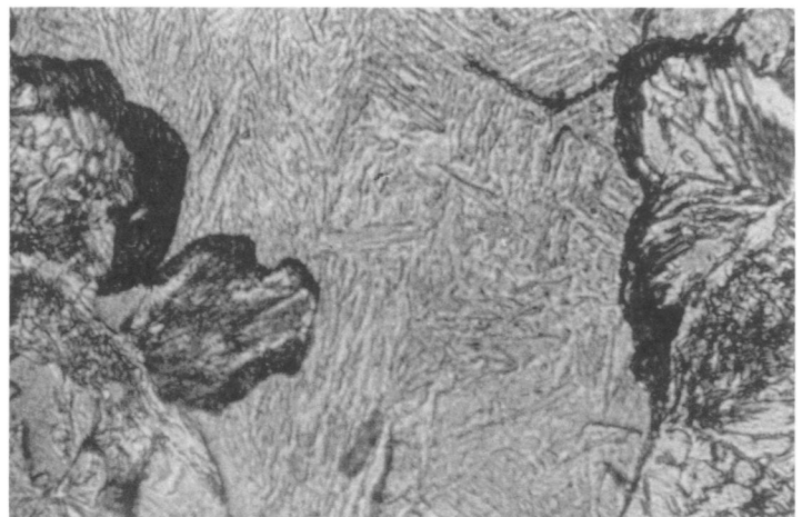
2f. Pearlite, surrounded by dark-etching material, in the midst of martensitic areas (possibly the result of a slow cool, forming pearlite in small areas, then a quench to transform the rest of the steel to martensite) × 1280
