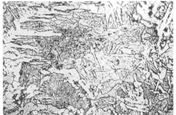
1b. Ferrite and partly spheroidized pearlite \times 320
