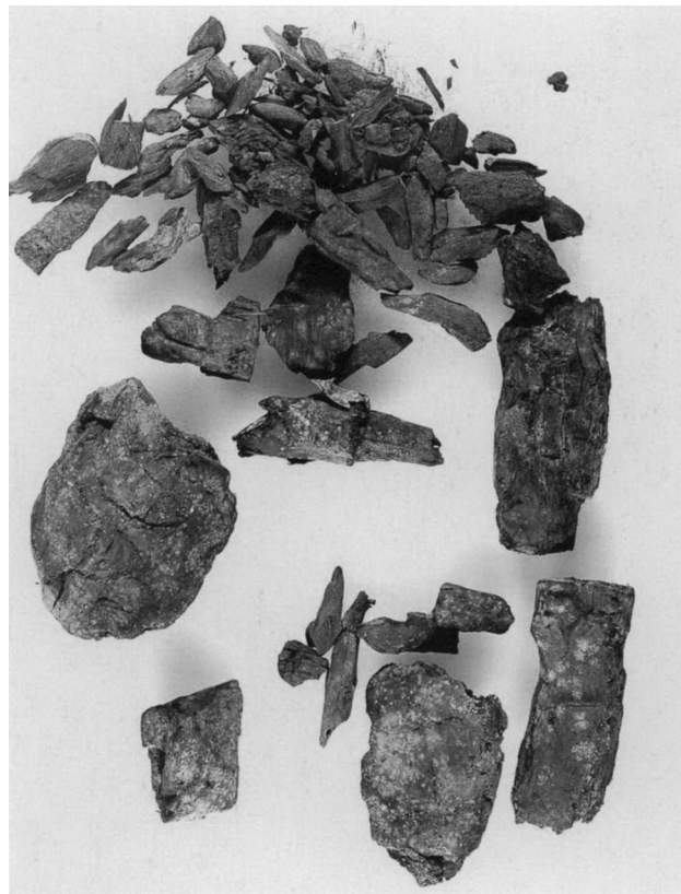
Figure 2a–b. Condition of wooden bases of Filippovka deer figures prior to restoration
