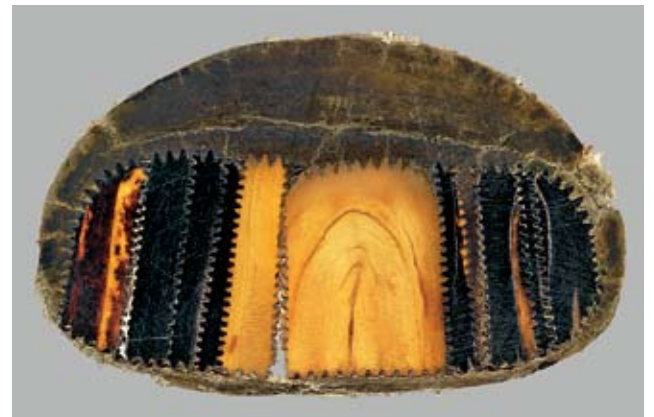
5. Cross section of a fifteenth-century composite bow. Whalebone or horn. The Metropolitan Museum of Art (X.800). The core of this bow does not contain any wooden backing like that in the bow of Figure 1 but is instead made up of layered strips of horn. The surface of each layer is deeply hatched or engraved with parallel lines (giving in profile a "toothed" appearance) in order to strengthen the bonding of the glued components. The same method was apparently employed for the inlays of horn, bone, and ivory in the stock.
