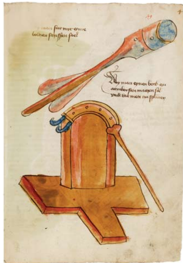
25. Johannes Bengedans. Büchsenmeister-Buch (see Figure 24), fol. 49r, showing at the top “How one shall shoot fire with a [crossbow] bolt,” and underneath it “How one shall make a [stationary] block for crossbows to span them with it”
