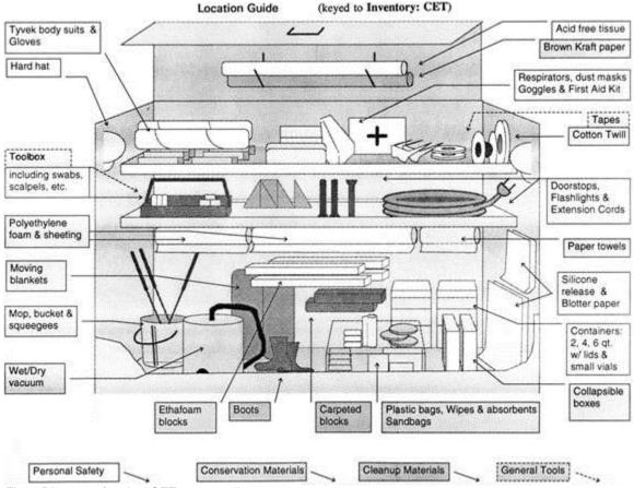
Fig. 1 Diagram of typical CET cart supplies.
