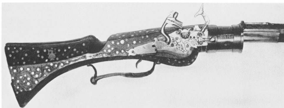
45. Detail of snaphance rifle with revolving cylinder by Pervusha Issayev and Ivan Romanov (stock maker), Russian (Moscow), 1625. Moscow, Kremlin Armory, inv. no. 7595 (photo: after Blackmore, Guns and Rifles of the World , fig. 564)
