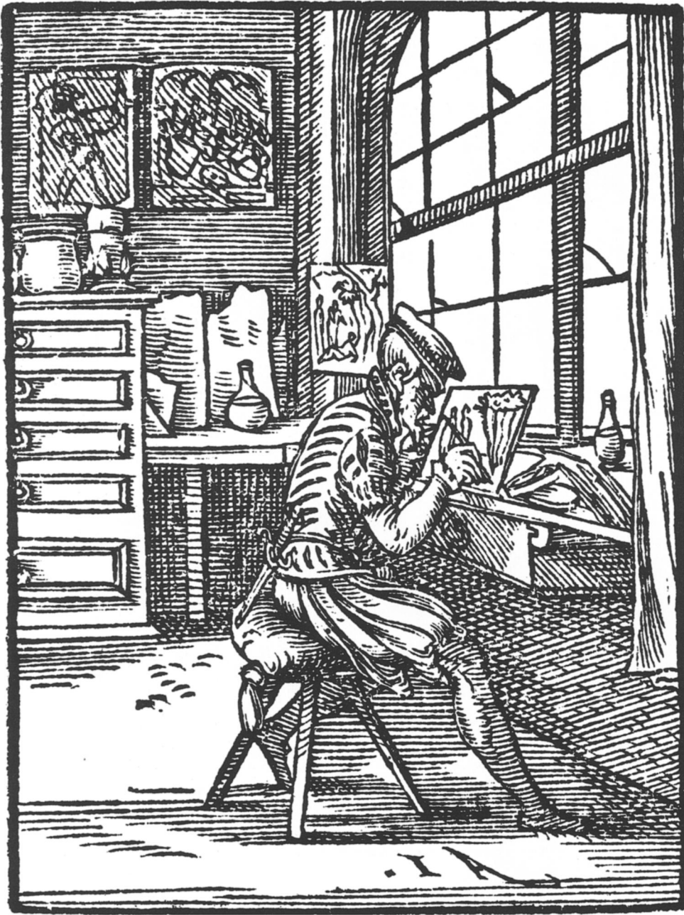
Figure 6: In the enameling process, a vitreous paste was painted on the surface of a sheet of white or clear glass. The sheet was then fired to make the enamel adhere, and care was taken to keep the temperature from going so high that the paint would flow beyond the confines of the design. Since the color was on the glass rather than penetrating it, the effect was less brilliant than in pot-metal glass (glass to which metallic oxides had been added during the molten state as coloring agents). Because of the low firing temperature, the enamel was quite unstable and frequently separated from the glass it decorated. The Glazier and The Glass Painter , woodcuts by Jost Amman. From Hartman Schopperus, " πανδηλία: Omnium illiberalium mechanicarum aut sedentariarum artium . . . " (Frankfurt, 1568), pp. 26, 25. Metropolitan Museum Library
