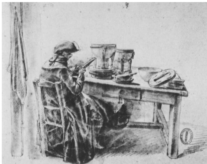
FIGURE 15. A répateur or garnisseur attaching supports to a pair of hemispherical bowls ( jattes rondes ), one of which is mounted on a turntable. His equipment includes a bowl of slip ( barbotine ) to serve as an adhesive and a brush for applying it. At the corner of the table is the open plaster mold from which the support in his hands was formed.
