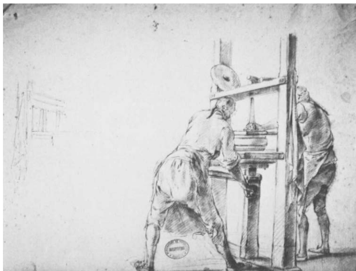
FIGURE 13. Mouleurs (molders) at a hand press, centering the mold for a plate in an early process ( moulage à pression ) that was slow and laborious. Deeper vessels were usually made on a kick-wheel (see Figure 11) or by pouring the porcelain paste ( pâte ) into molds consisting of multiple parts. Drawing, third quarter of 18th century.
