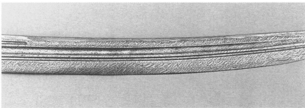
Figure 13. Detail of blade of Figure 12, showing huawengang pattern (photo: author)
