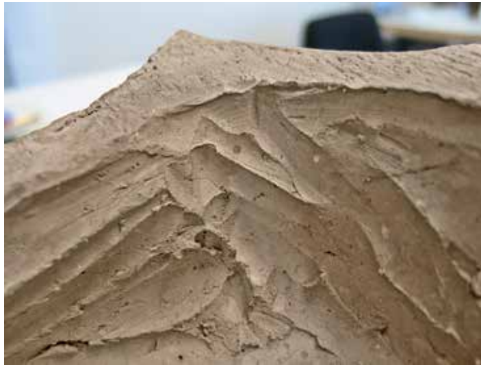
fig. 9 (a) Finger marks from pressing soft clay into the mold; (b) Fingerprints found on the back of the lunette
