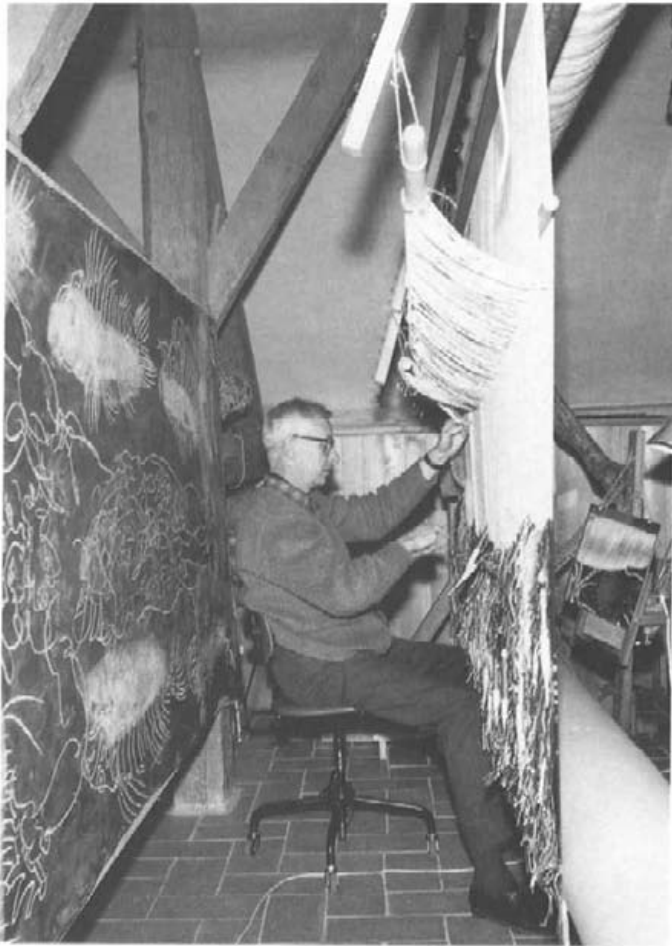
Fig. 5. A tapestry weaver working at a high-warp loom. The finished web fills the lower part of the unrolled warp. The cartoon hangs behind the weaver. He faces the back of the growing fabric and can see the front of it reflected in the mirror placed before, and just above, the lower beam.
