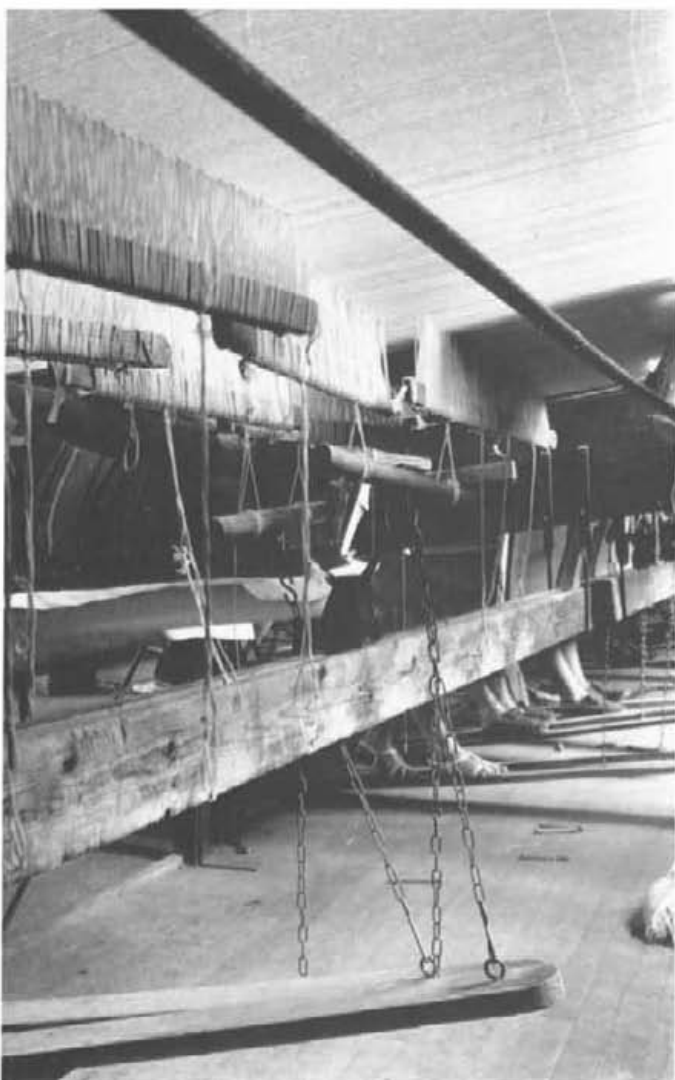
Fig. 11. A weaver working at a high-warp loom. The various bobbins he uses, each of which carries weft yarn of a different color, hang from the edge of the web on the back of the growing tapestry. The heddles through which every other warp yarn passes hang from rods suspended just above the weaver's head.
