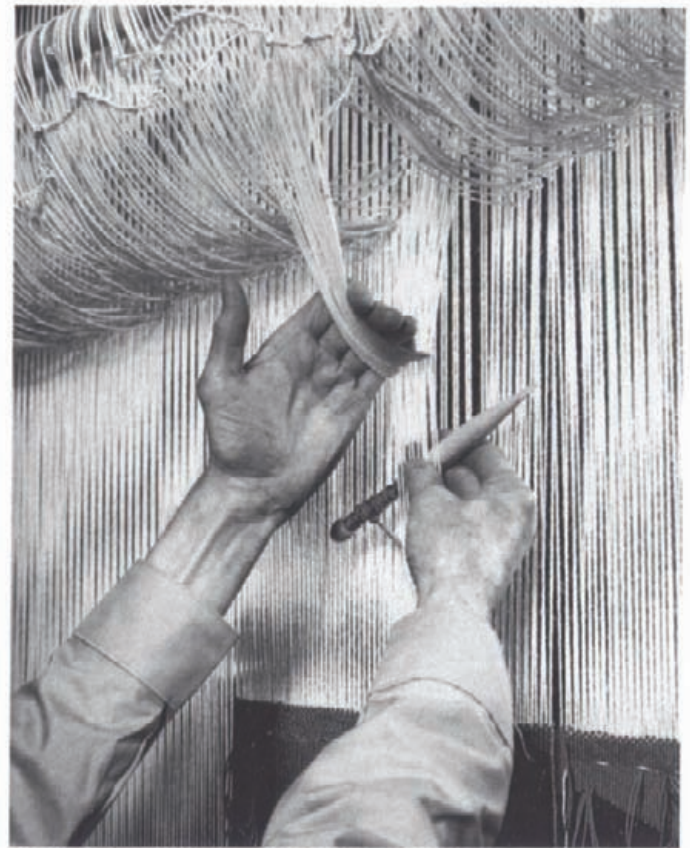
Fig. 9. A weaver working at a high-warp loom opens the second shed by pulling on some heddles; this brings the warp yarns in the farther plane to a position in front of the yarns in the nearer plane, and the weaver passes the bobbin through the shed from left to right.
