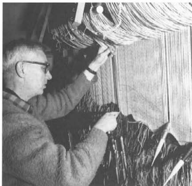
Fig. 10. The tapestry web begins to form. The weft yarn has passed with the bobbin through two sheds, in front of one set of warp yarns and behind the other.
