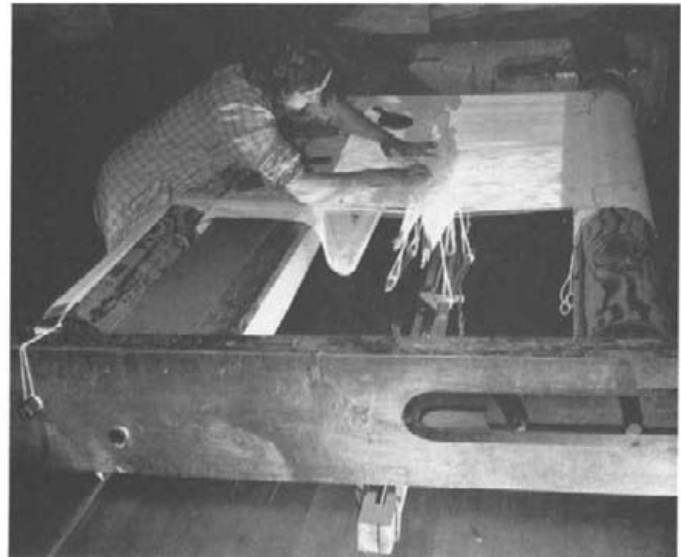
Fig. 6. A weaver working at a low-warp tapestry loom. The warp is stretched horizontally between the front and back beams. The cartoon lies under the warp and is supported on a board that extends across the loom next to the front beam.
