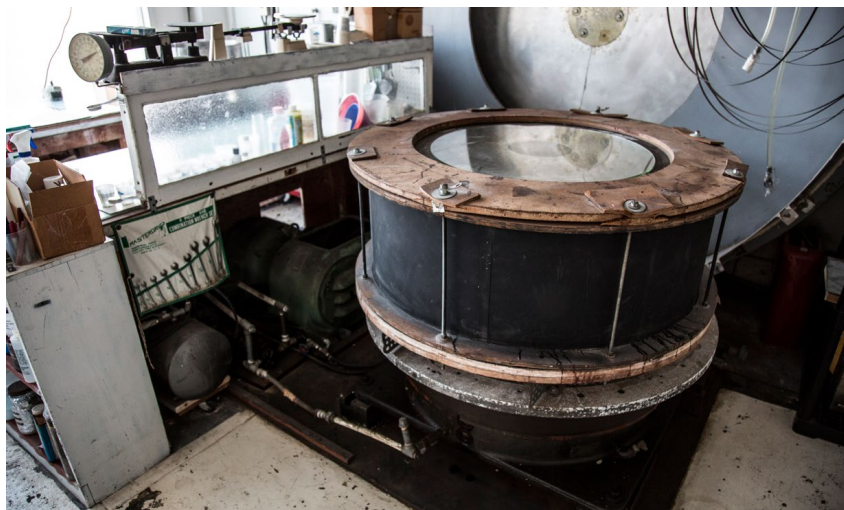
[Fig. B] Centrifugal vertical spin-casting mold tool (diam. 40 in.), 1971. Eversley reused a 1936 turntable to create this tool to produce his parabolic sculptures.
