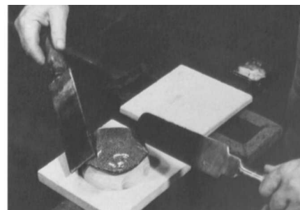
Slumping Fig. 27. The soft disk is transferred to a slumping form.
