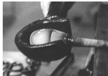
Blocking Fig. 46. A water-soaked wooden mold, known as a block, can be used instead of the marver (figs. 31–33) to give a gather of glass its initial shaping. The block is lifted firmly against the glass as the blowpipe is slowly turned.
