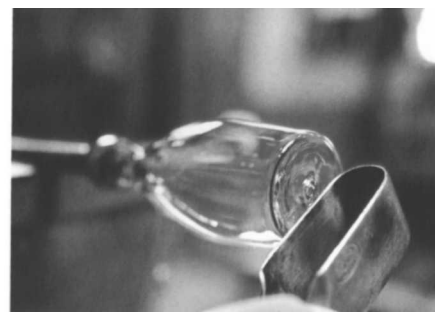
Fig. 74. Having been reheated to slightly soften the glass, the bottom is forcefully pushed flat.
