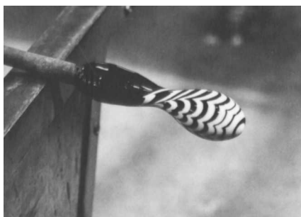
Fig. 84. The bubble is blown larger, and a broad constriction is formed in the glass near the blowpipe (figs. 37, 38) as the glassblowing process is continued.
