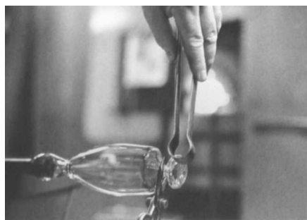
Fig. 72. The constriction is held tightly with shears to both weaken and chill it. Tweezers are brought into position to break away the outermost part of the glass.
