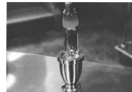
Dip-Molding with a Diamond-Patterned Mold Fig. 34. After the glass has been inflated by blowing, it is lowered about three-quarters of the way into a dip mold (the upper part remains outside the mold).
