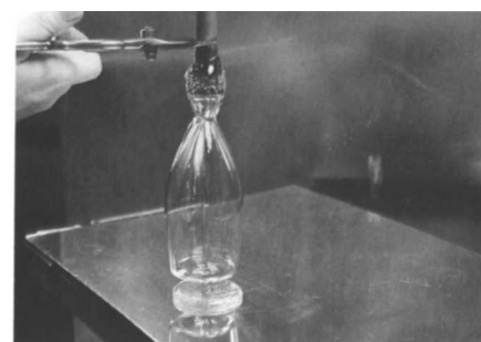
Fig. 77. The still-hot vessel is lowered onto the soft disk.
