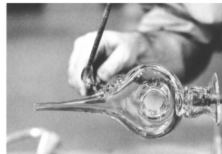
Fig. 69. The thick thread of glass is tooled and pressed against the shoulder to create the decorative pattern. Finally, the glass is cut free of the metal rod, and the finished object is broken from the pontil and placed into the annealing oven for slow cooling.
