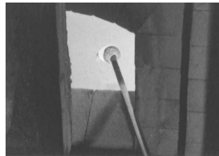
Marvering Fig. 30. Hot glass is gathered from a furnace on one end of a long metal tube called a blowpipe. Inside the furnace, the glass is maintained at a temperature of roughly 2,000°F (1,093°C).
