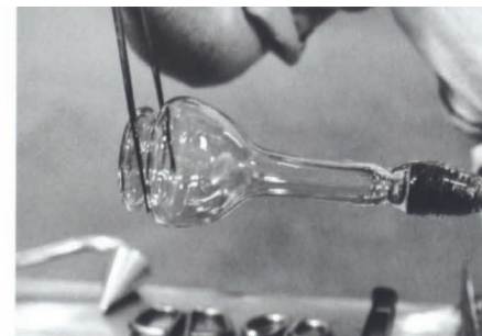
Making a Roman Foot Fig. 50. A constriction (neck) is formed near the bottom of the bulbous vessel body.
