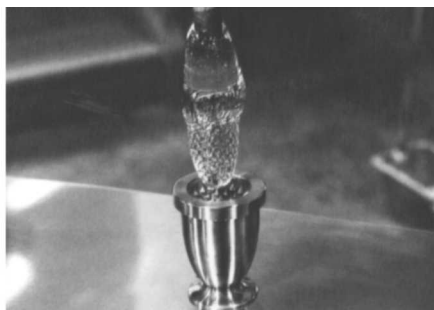
Fig. 36. When the glassworker deflates the bubble slightly by sucking a little air out of the blowpipe, the glass pulls free of the undercuts in the mold and can be removed.
