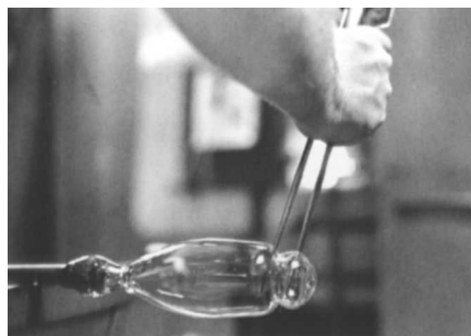
Fig. 70. A constriction (neck) has been formed near the blowpipe in a bubble of inflated glass (figs. 37, 38). Another constriction is begun using the jacks near the tip of the elongated bubble.
