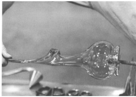
Fig. 55. The neck and rim of the sprinkler bottle are given their final form by pulling the edges of the soft glass downward and then rapidly upward.
