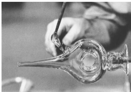
Fig. 68. A bit of glass freshly gathered from the furnace at the end of a metal rod is fused to the vessel's shoulder and then pulled away slightly to form a thick thread.
