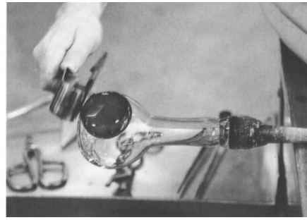
Fig. 81. The colored glass is pressed flat. The glassblowing process continues until the vessel is completed (see figs. 50–55, for example).
