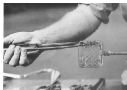
Fig. 43. More reheating follows, and the vessel is given its final shaping. When cool enough to hold its form, the finished object is broken off from the pontil and placed in the annealer for gradual cooling to room temperature.
