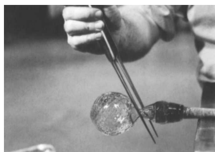
Fig. 38. After more inflation, the neck is made narrower.
