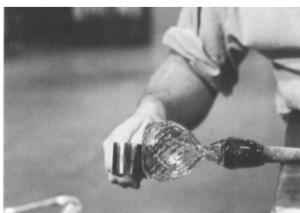
Flattening the Bottom Fig. 39. Following reheating to soften the end of the bubble, the base of the object is formed.
