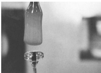
Cane-Making Fig. 20. Successive gathers of contrasting-colored glasses have been built up on the end of a metal rod. On another rod, a thick disk of colorless glass has been formed and allowed to cool and stiffen.
