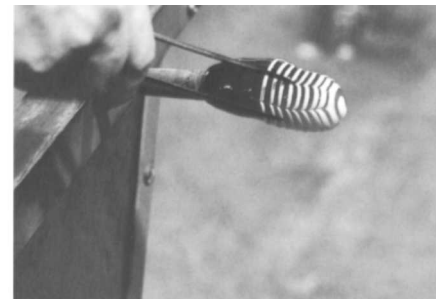
Fig. 83. After the bubble is reheated, combing begins. A pointed tool is dragged up the softened surface, pulling and distorting the spiral thread of white glass.
