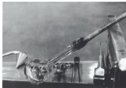
Fig. 49. Because it is thin walled, the tube thus formed cools quickly. The thick glass at its tip stays soft and can be rapidly inflated.
