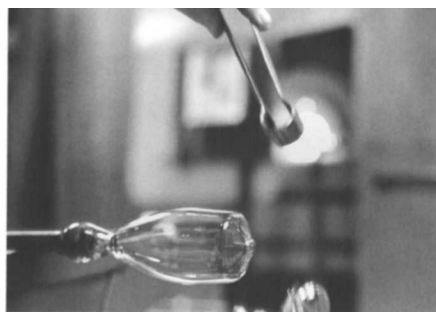
Fig. 73. A sharp tap on the end of the glass cleanly breaks the tip away, leaving a hole in the end of the bubble.
