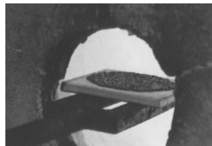
Fig. 25. The plate (in this case a piece of ceramic kiln shelf) is placed in a furnace or kiln.
