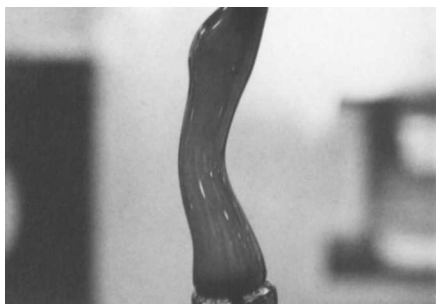
Fig. 22. The two rods are pulled in opposite directions, elongating the soft glass.
