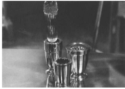
Fig. 44. Unlike the diamond-patterned mold shown in figures 34 to 36, a mold with vertical ribs has no undercutting that would require shrinking the bubble of glass to release it from the mold.
