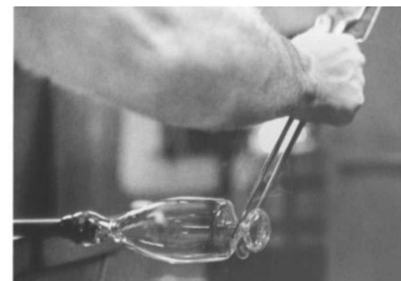
Fig. 71. The constriction is made narrow but not squeezed to the point where the passage between the two parts is closed off.
