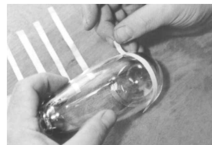
Fig. 85. Strips of gold leaf on a paper backing are attached in patterns to the surface of a cooled tubular glass blank. A mixture of water and gum arabic is frequently used as an adhesive.
