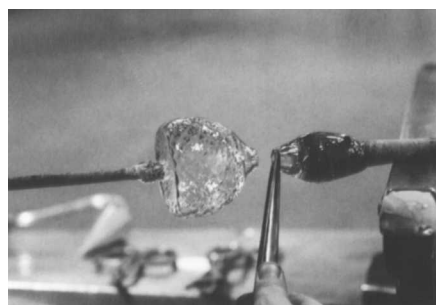
Fig. 41. The glassworker delivers a thermal shock to the neck by squeezing it with the cool pincers and at the same time taps forcefully on the blowpipe, causing the neck to break.
