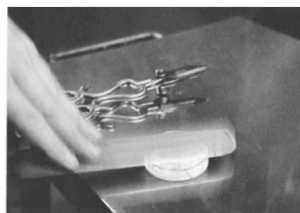
Fig. 76. The gob is flattened with a tool to form a disk.
