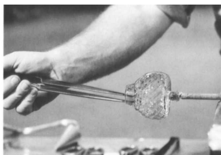
Creating a Rim Fig. 42. After the object is reheated, the jacks are used to widen the hole left by the blowpipe.
