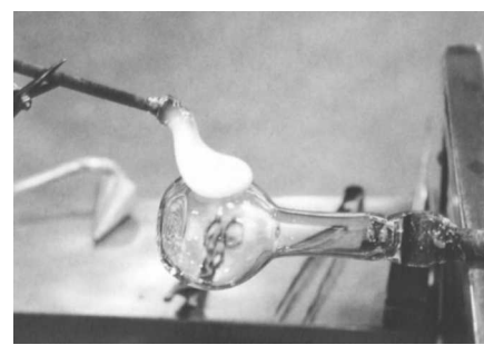
Fig. 79. A flattened mass of colored glass freshly gathered from the furnace is placed on the side of a partially completed vessel made of colorless glass.
