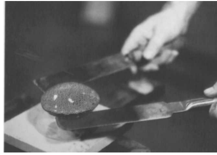
Fig. 29. When it has cooled enough to become hard, the glass object is pried free of the form and placed in an annealing oven for slow cooling to room temperature.
