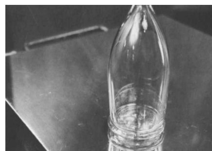
Fig. 78. Vessel and disk are firmly pressed together, creating a permanent bond. The glassblowing process is continued to complete the tumbler as in figures 40 to 43.
