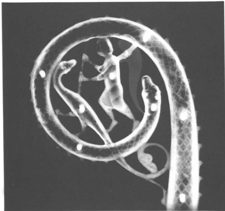
Fig. 24. X-ray of the crosier head (cat. 109) reveals the porous texture of the solder along the single vertical seam that joins the two halves of the crocketing, the volute, and the figures of Saint Michael and the dragon. (Photo: Pete Dandridge)
