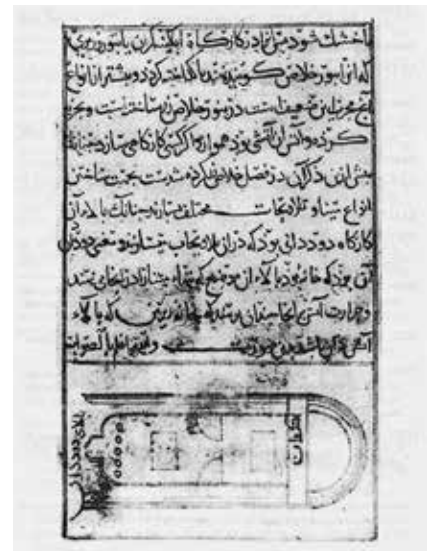
Fig. 72. Reproduction of a kiln employed for enamel ( mina ) and luster ( talavih ) in the Jawahirnama-yi Nizami of Nishapuri. Malek Library, Tehran (MS 3609; fol. 153v)
