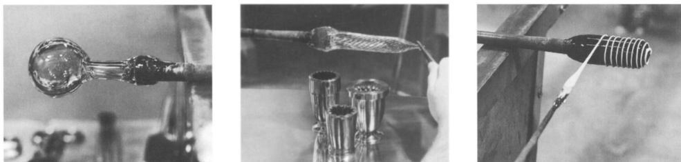
Figure 1 Three examples of hot-working, performed by William Gudenrath in the Studio of the Corning Museum of Glass: inflating a gather of glass; twisting glass that has been dipped into a ribbed mold, so as to create a spiral pattern; and threading soft white glass around a darker bubble
