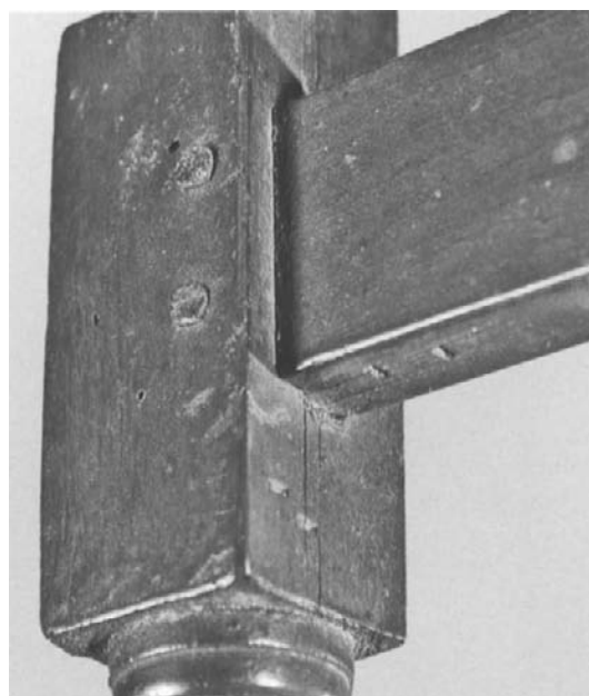
Fig. 87, cat. no. 58. Joiner's assembly marks.
