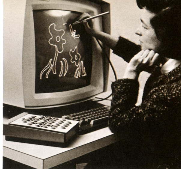
1. Freehand drawing on the CRT's screen with the light pen. The table of commands is at the left; the keyboard beneath the screen is used to enter written and coded information into the computer and CRT
