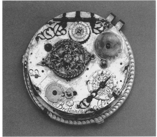
Figure 34. Auguste Bretonneau (French, recorded 1638–58). Movement of the watch in Figure 33, with a late-seventeenth-century balance spring and balance bridge. Gilt brass; steel, partly blued; and silver, diam. of back plate 3 3/4 in. (8.2 cm)
