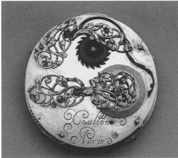
Figure 32. Jacques Goullons (French, recorded 1626–d. 1671). Movement of the watch in Figure 10. Gilt brass and steel, partly blued, diam. of back plate 1 7/8 in. (4.9 cm)
