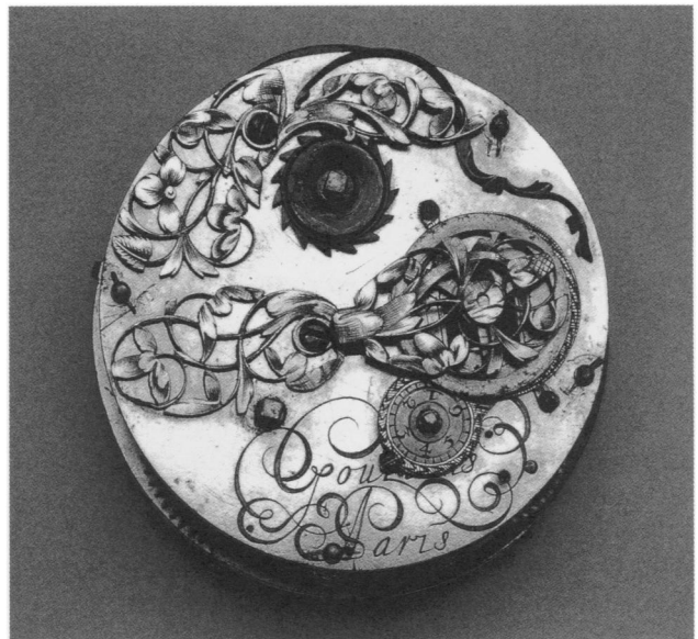
Figure 31. Jacques Goullons (French, recorded 1626–d. 1671). Movement of the watch in Figure 3. Gilt brass; steel, partly blued; and silver, diam. of back plate 2 in. (5 cm). The balance spring and the figure plate used to regulate it are later additions
