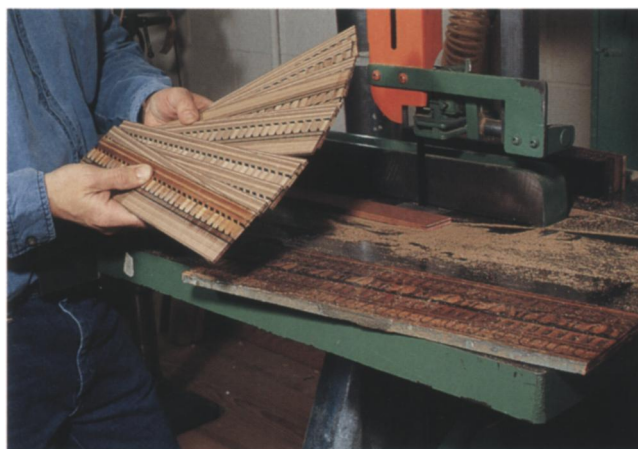
Fig. 31. A block of toppo intarsia about two inches thick and one foot long can produce about twelve feet of the same design.
