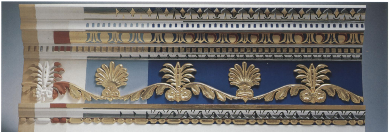
Fig. 18. Reconstruction of cornice section in which the working methods of 15th-century craftsmen have been re-created. From left to right: poplar base, gesso layers, bole and gilding, underpaint, and, from middle to right edge, as completed
