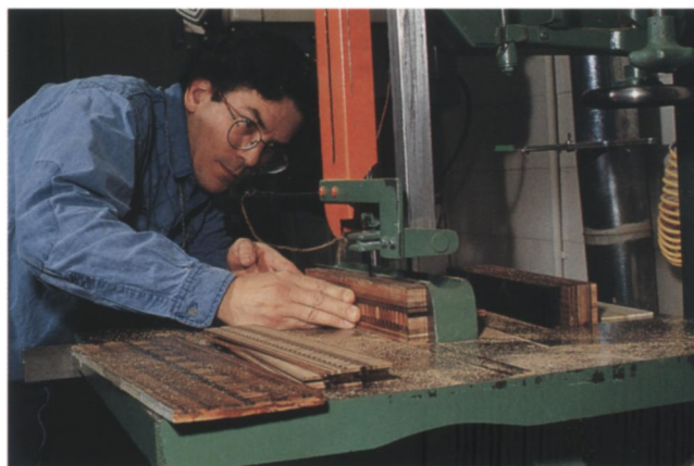
Fig. 30. Sawing a block of toppo intarsia into slices approximately \frac{1}{8} inch thick
