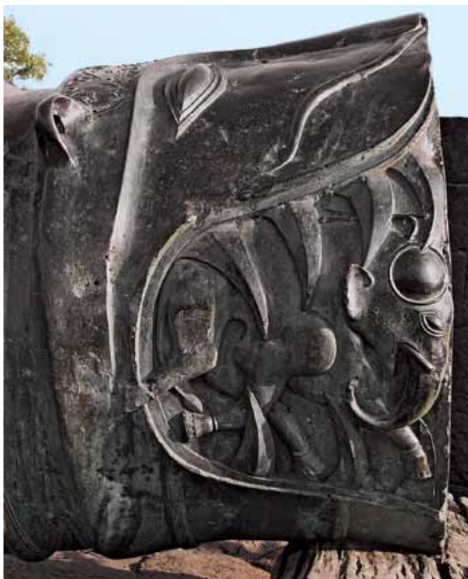
Fig. 4. “Malik-i Maidan,” bronze cast bombard, made at Ahmadnagar, 1549, now mounted at Bijapur Fort. A century after gigantic guns had been discarded in Europe, they were successfully introduced to the Deccan.
