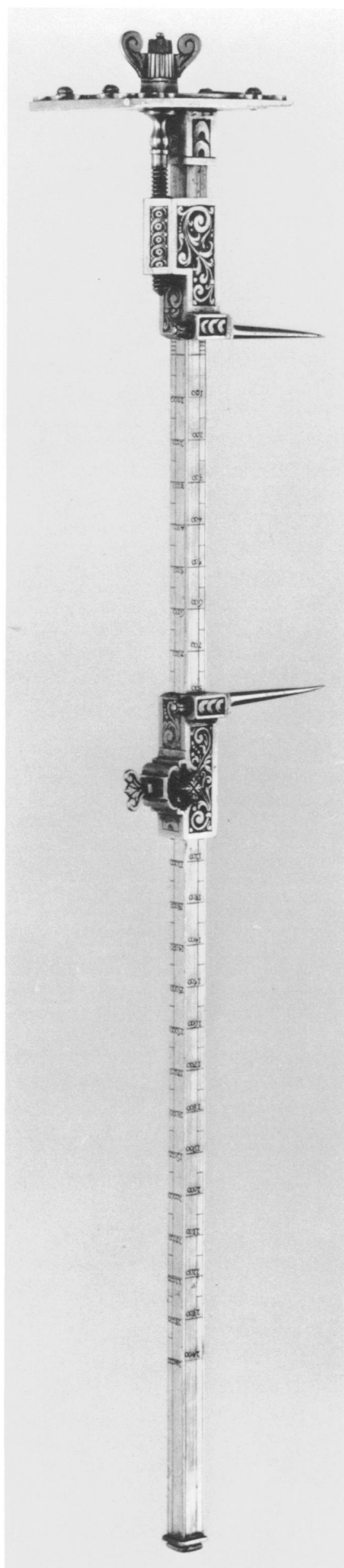
12. Detail of Figure 9 showing the subdivisions of the basic unit of the measurement scale
